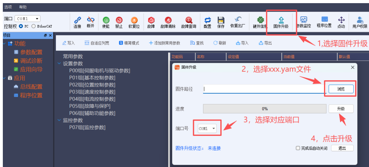
图 3-24 串口升级方法 Figure 3-24 Serial Port Upgrade Method
